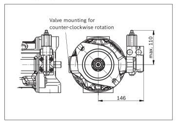
**▼ DRG - Pressure controller, remotely controlled**
