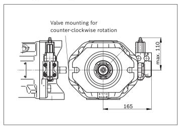
▼ DRG - Pressure controller, remotely controlled
