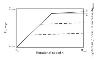
Characteristic curves valid at  $n_1 = 1500$  rpm and  $\vartheta_{fluid} = 50$  °C.
