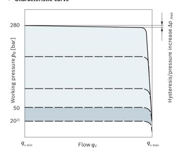
Characteristic curve valid at  $n_1$  = 1500 rpm and  $\vartheta_{fluid}$  = 50 °C.
