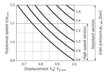
During continuous operation in overspeed over  $n_{\text{nom}}$ , a reduction in operational service life is to be expected due to cavitation erosion.
