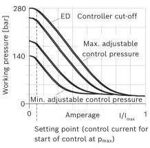
► Hysteresis static current-pressure characteristic curve < 3 bar.
