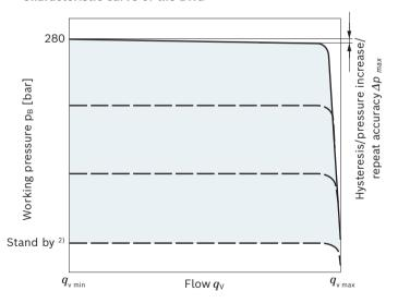
Characteristic curve valid at  $n_1 = 1500$  rpm and  $\vartheta_{fluid} = 50$  °C.
