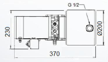
The 12V DC single-acting power pack is suitable for all single-acting applications and ideal for use in the following applications:
