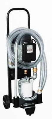
The hydraulic filtration system removes solid contamination and water from petroleum based fluids such as hydraulic fluid and gear and lube oils. The filter cart can be used to pre-filter fluids, transfer fluids or to clean existing systems.
