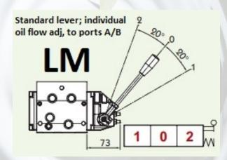
Type L— with no adjustment facility—Type LM with adjustment in front, to regulate max level.
