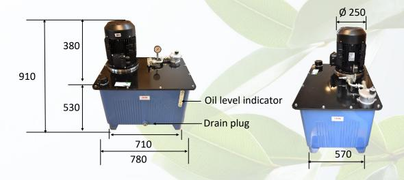
This Hydraulic Power Unit comes with a double pump at 8+8 cm3 with high/low function.
